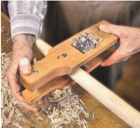
▲ Pic. 5 Jeff's rounded-sole trapping plane uses parts sawn from a metal spokeshave
